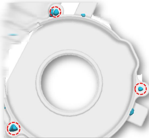
Shrinkage risk was observed in pre-simulation results.
