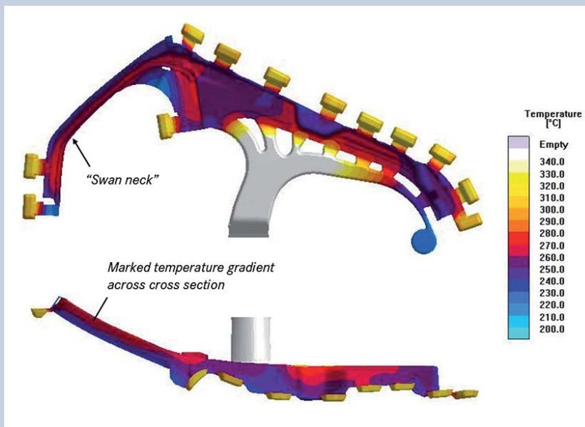
Temperature distribution in the casting and in the gate after ejection.
