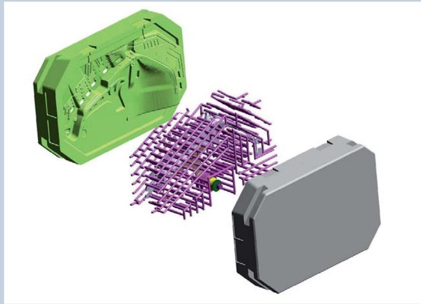
CAD model of the casting including runner system, cooling and heating channels and the two die halves
