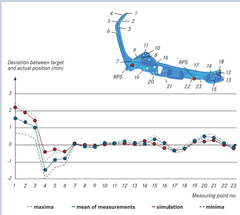
Calculated versus measured distortion after clipping
