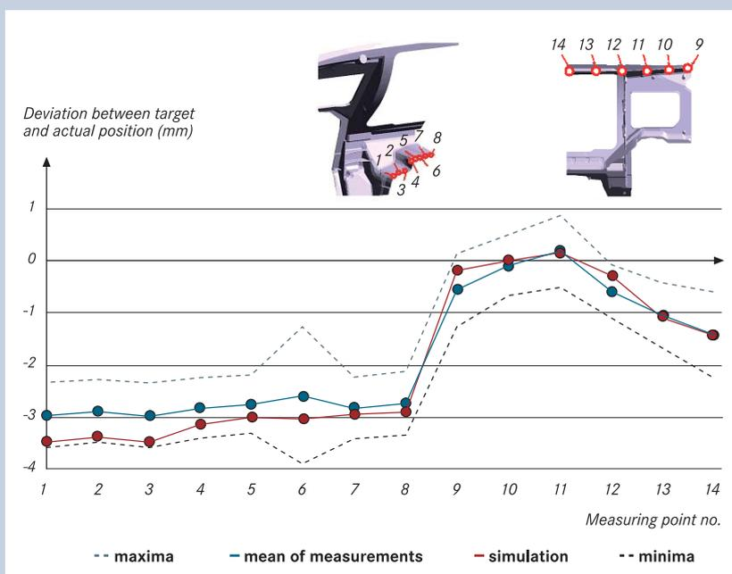
Calculated and measured distortion of the bulk head after heat treatment
