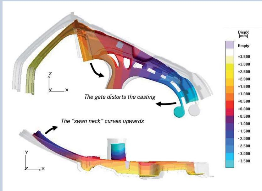
Deformation of the casting after cooling down. For illustration purposes the deformed and non-deformed geometries of the casting are shown.
