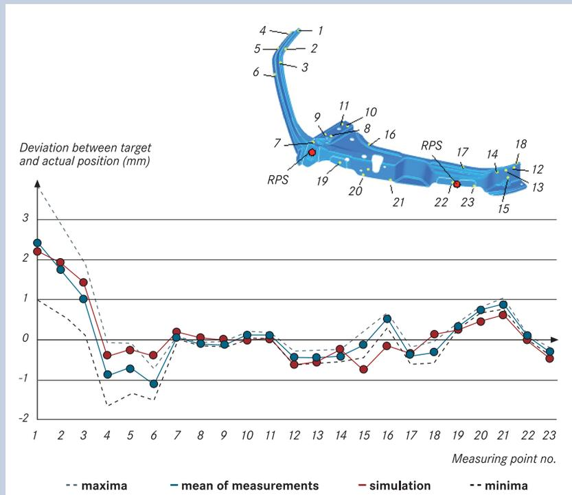
Measured versus calculated deviations from the target geometry for 23 measuring points of the door lock panel
