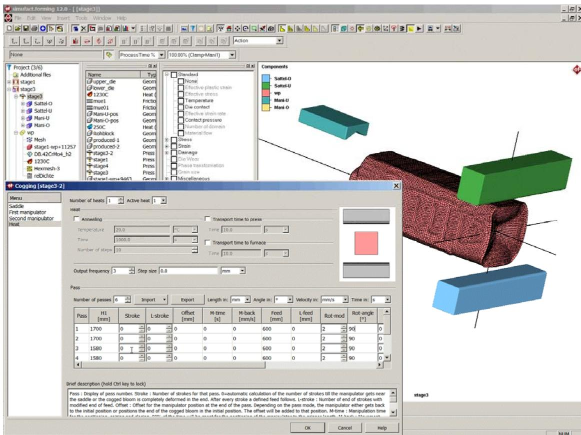
Fig. 2: The model of the cogging simulation
