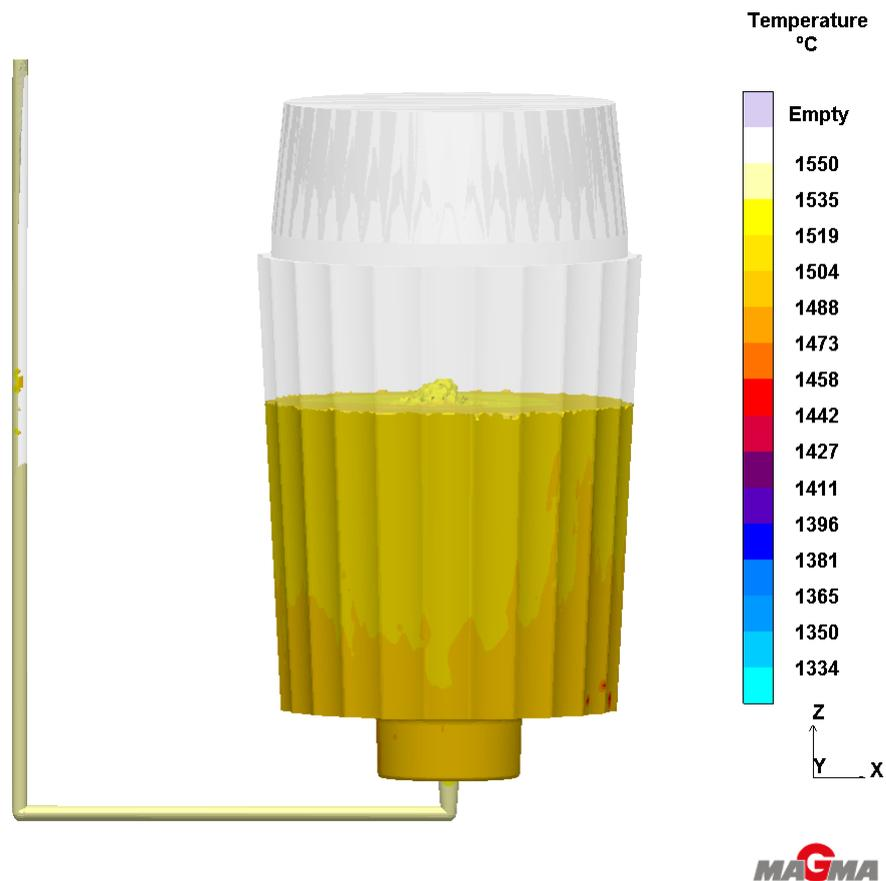
Fig.1: Simulated temperatures after 15 minutes of teeming
