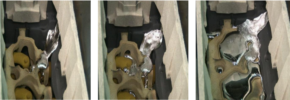
Fig. 3: Change in flow direction during the mold filling process of a cylinder head. The cover core was modified to allow high-speed videos of the melt flowing from the runner through the gates to be taken.
