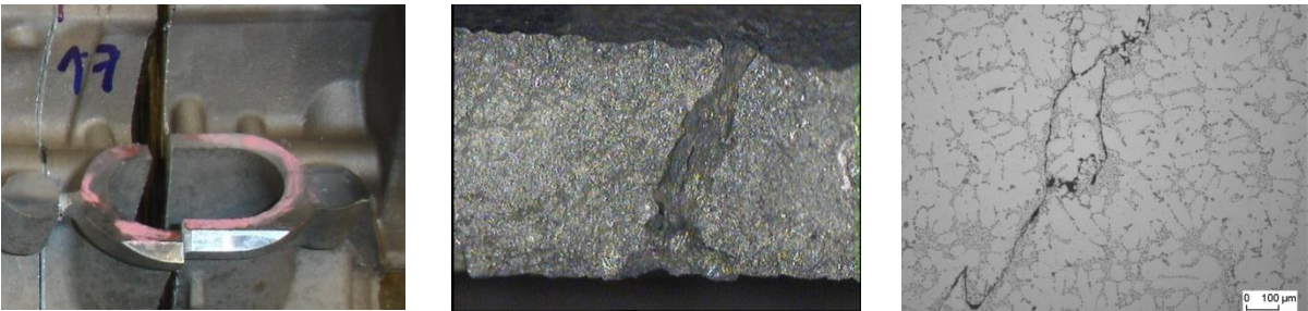
(a) Cut through leaking cylinder head (b) Fracture analysis through leaker (c) Microstructure analysis
