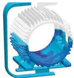
Entrapped gas with the original (top) and optimized (bottom) gating system
