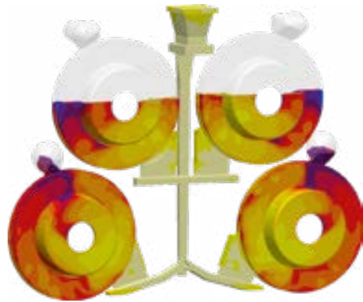
Mold filling of four gray iron brake discs
