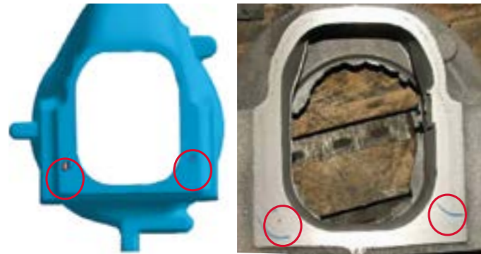
Porosity in a ductile iron housing
