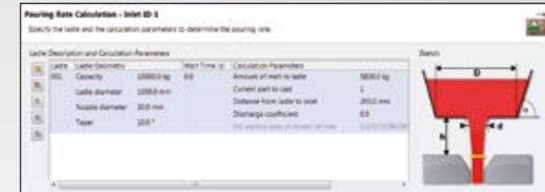
Outflow from the bottom pour ladle - calculated from ladle geometry and current melt quantity
