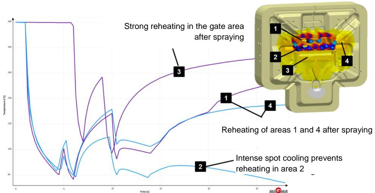
The temperature curves in the die area close to the surface illustrate the effectiveness of the spraying process combined with the internal die thermal control. The internal spot cooling in area 2 locally removes energy from the die and reduces the reheating of the die surface.
